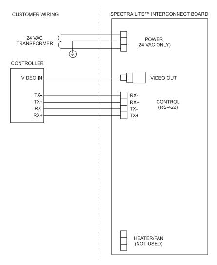
Figure 9. Wiring Diagram for Spectra Lite™
